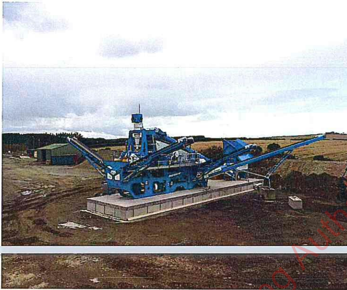
Photograph 2.1: Image of a typical washing and screening plant
